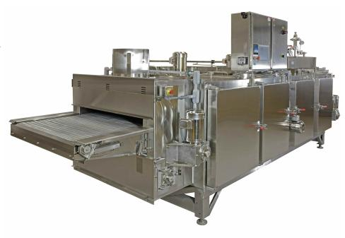
heat transfer where internal freezer temperature can reach as low as -150°F (-101°C) depending on cryogen used. Conveyor speed and freezer temperature can be adjusted for maximum processing flexibility. Automatic temperature and pressure control systems adjust cryogen injection to accommodate variations in product load and temperature variations.
