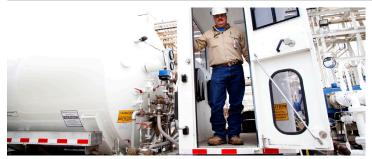
Nitrogen is the most widely used gas for purging and inerting operations, due to its cost effectiveness, availability, and non-hazardous effects. Linde Services Canada Inc. uses nitrogen to safely purge potentially explosive hydrocarbon and air mixtures from vessels, transfer lines and equipment, leaving an inert atmosphere for shutdown and start up activities.
