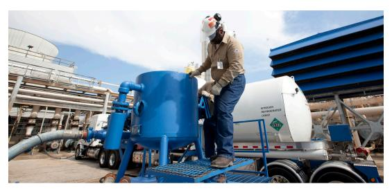
Linde Services Canada Inc. provides fast and economical pipeline cleaning that dries, cleans and inerts in a single operation.
